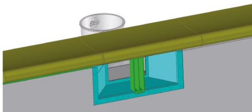
Only remove the support column from the skimmer mouth when the mortar is completely set
