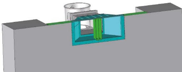
Position the welded mesh, making sure that the ends coincides with the pool chaining
